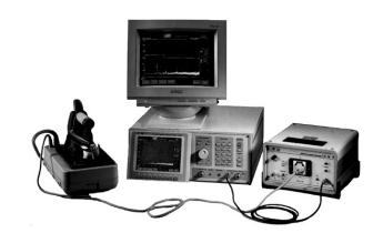
The "action" feature, for example, provides functionality of a complete automatic system without the need for an external PC. It can control LISNs, perform a sequence of measurements, find the worst case reading and print or save the desired results. This may be programmed, stored and then repeated, completely automatically, as many times as are needed with no need for an attending operator. The built-in hard disk and 3 ½ inch floppy drive give extra convenience to save, load or transport data.
